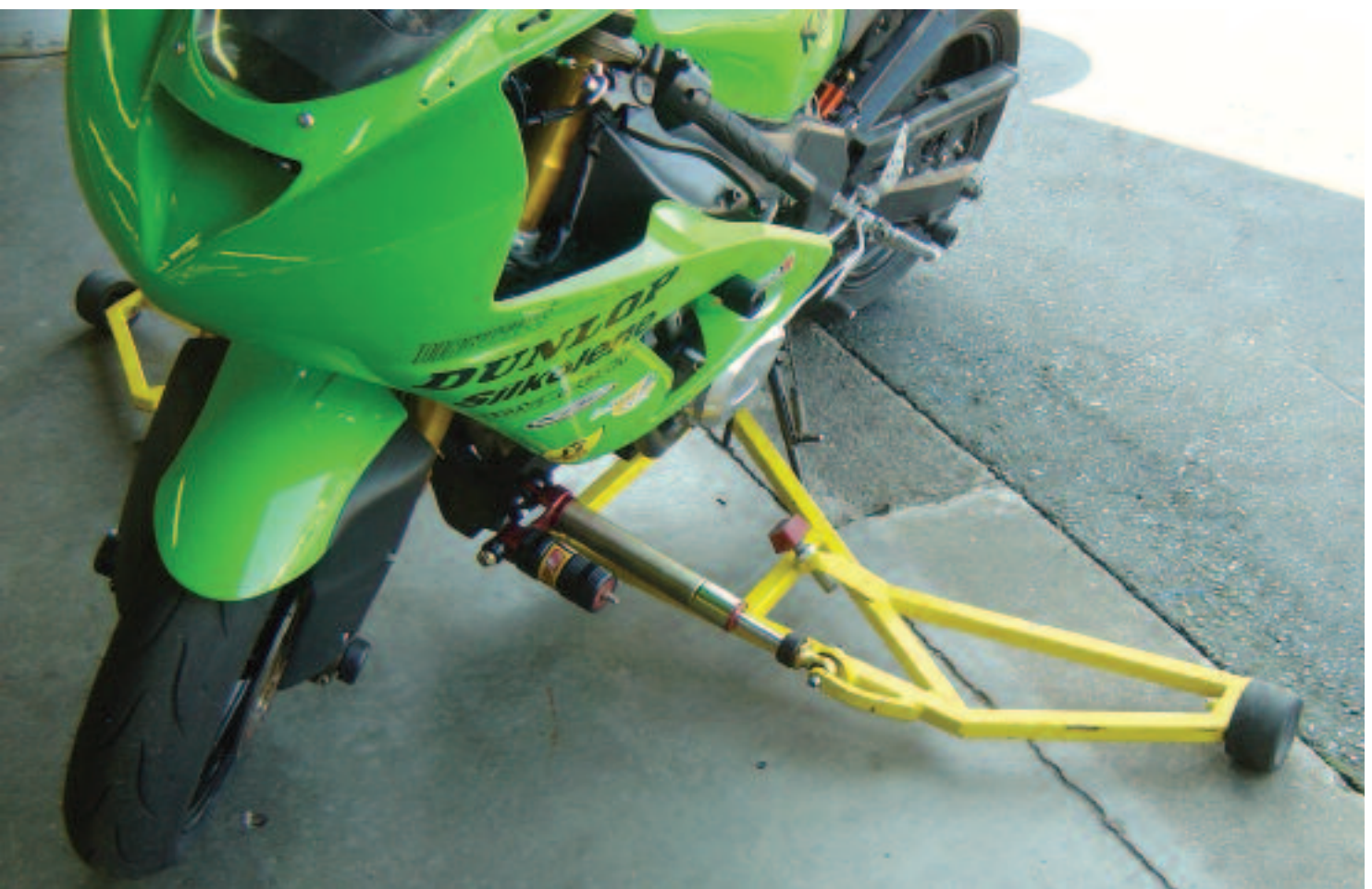
ABOVE The lean and body positioning bike with hydraulically damped out-riggers. Unfortunately out of action during the course days (Tony Foale)
