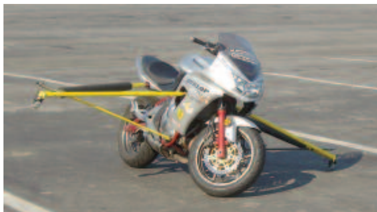
ABOVE The lean and body positioning bike with hydraulically damped out-riggers. Unfortunately out of action during the course days (Tony Foale)
