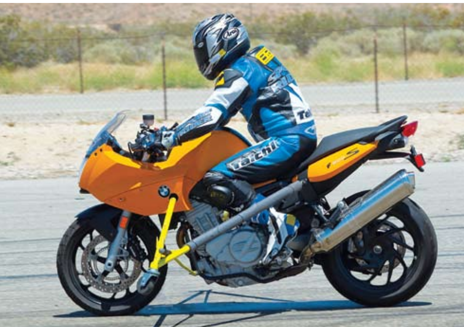
The panic braking bike—a BMW F800 S with outriggers to keep it from tipping over—allows students to understand what it feels like to get up to and past the point of front wheel lockup (note the tire smoke trail from the front tire). This helps break through what Code terms one of the many “barriers”; survival instincts that keep us from exploring our potential as better riders.
